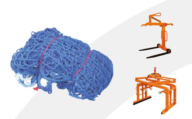
The CS0003 Safety Restraint Net has been designed specifically for use with crane forks and block grabs. The net is designed to restrain the load on the equipment and must be gathered as tight as possible around the lifted load to maximize effectiveness. The net is not designed to catch a falling load.
